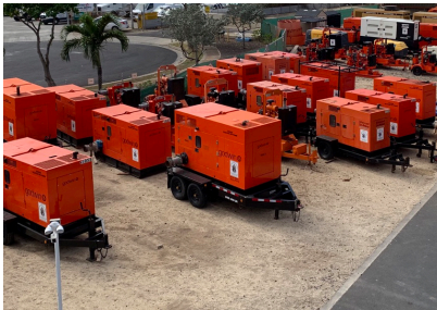
Dri-Prime Pumps for Sewer Bypassing & Dewatering
